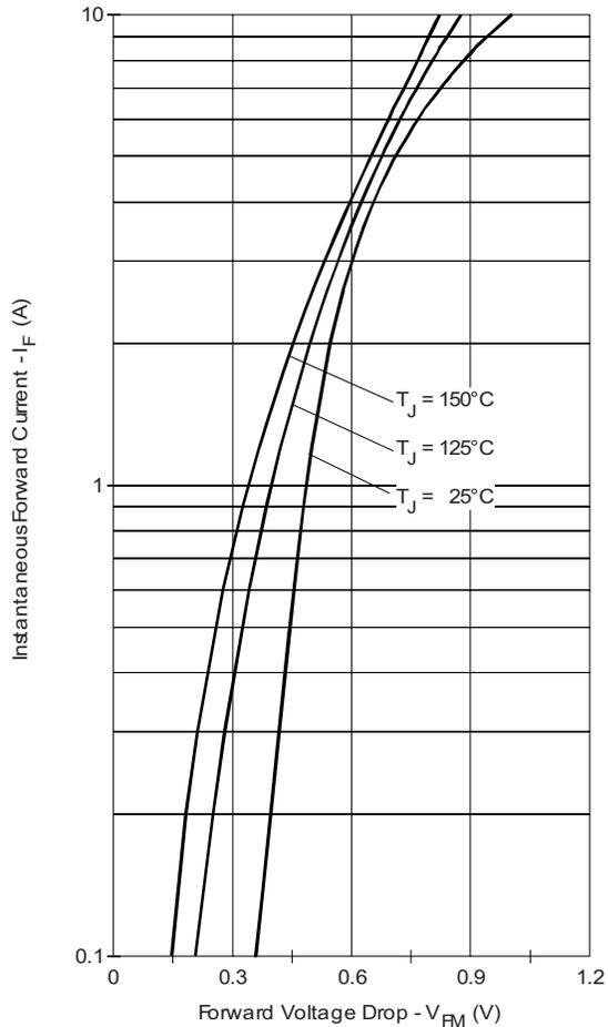
Fig. 1 - Maximum Forward Voltage Drop Characteristics
