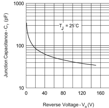
Fig. 3 - Typical Junction Capacitance vs. Reverse Voltage
