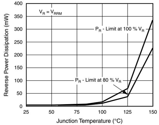
Figure 4. Max. Reverse Power Dissipation vs. Junction Temperature
