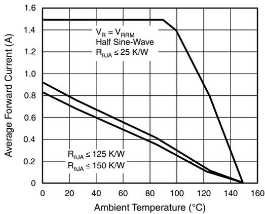
Figure 2. Max. Average Forward Current vs. Ambient Temperature
