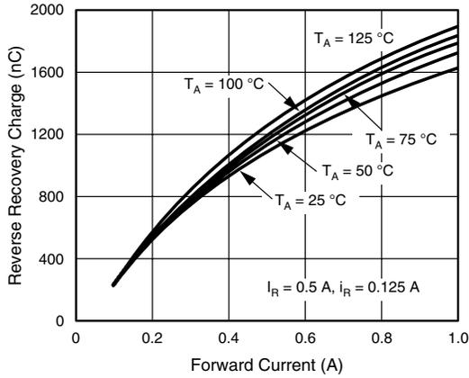
Figure 7. Reverse Recovery Charge vs. Forward Current
